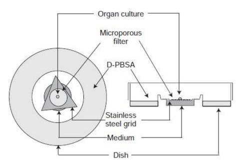
Figure 1: Organ Culture Small fragment of tissue on a filter laid on top of a stainless steel grid over the central well of an organ culture dish
