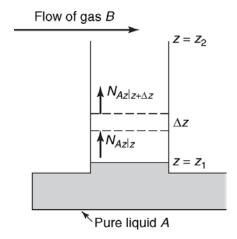
Consider the control volume S  $\Delta$  z, where S is the cross sectional area of the tube. Mass balance on A over this control volume for a steady-state operation yields
