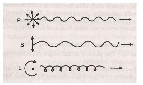
**P-waves (primary or push and pull waves**): - These are high frequency short wavelength longitudinal compressive type, like sound waves. These take the quickest path and are transmitted by oscillations in the direction of propagation. P-waves travel through solids, semi-solids and liquids, i.e the crust the mantle and the core of the earth at speeds 5 to 15km/s
