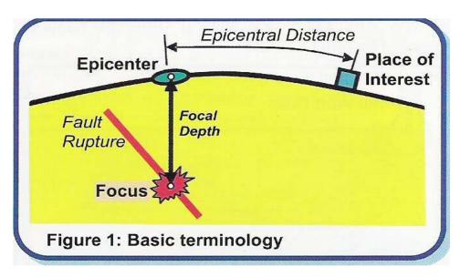
An earthquake is the vibration of the earth produced by the rapid release of energy. Although earthquake occurs occasionally, but destruction they cause through loss of life and property. The exact spot underneath the earth surface at which an earthquake originates is known as its **FOCUS**, while the point on the earth surface lying above the focus is defined as the **EPICENTRE**.
