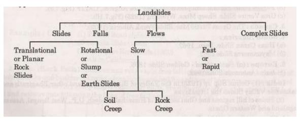
**SLIDES**: - Sudden downhill movements of rock and or unconsolidated rock material on a definite identifiable water lubricated or not down slope inclined plane called a shear or slip plane between the separating and remaining masses. The slip plane may be a bedding plane, joint plane, fault plane, and schistose or cleavage plane.
