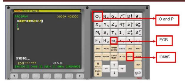
In program panel press letter in smaller font press **Shift** then press button for example to type letter p press **Shift** then press **O and P** Button. After entering one line of code press **EOF** button press **Insert** button add this code to numerical control panel.
