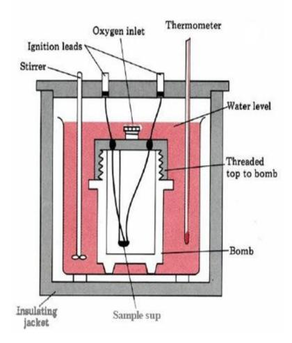
Fig. Bomb Calorimeter
