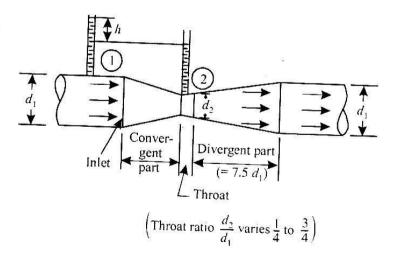
SCHEMATIC DIAGRAM OF VENTURIMETER
