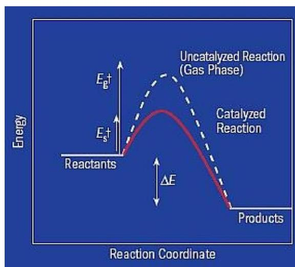
Figure 2. Potential energy surface illustrating how catalysts reduce the activation barriers of reactions.
