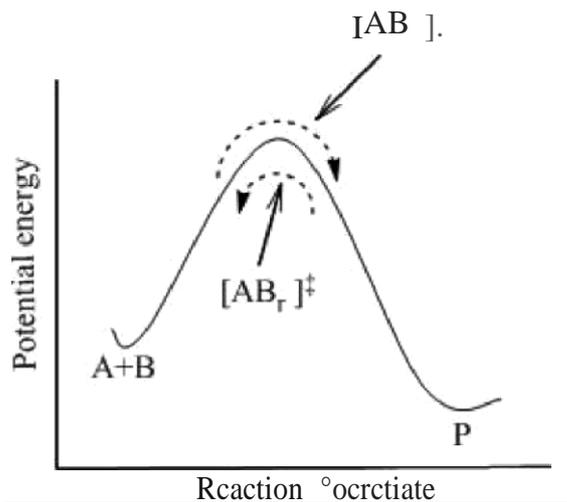
Activated complexes are highly unstable and are not observed *because they* are unstable. The activated complex is the point in a reaction where its **potential energy** is highest.
