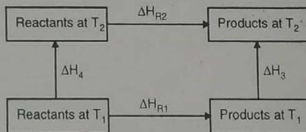
Fig. 6.1 : Effect of temperature on heat of reaction
