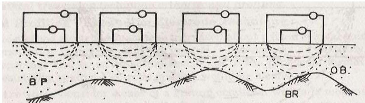
**Fig. 16.30. Horizontal profiling - Lateral Traversing Technique.**
