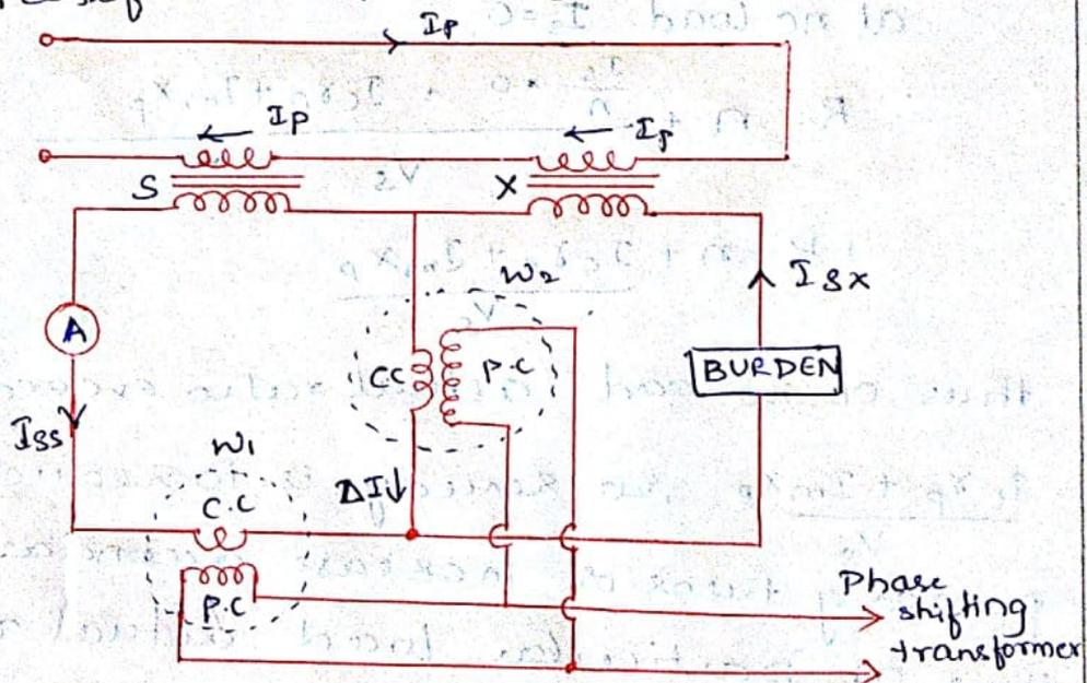
\* Two transformers (X & S) primaries are connected in series.
