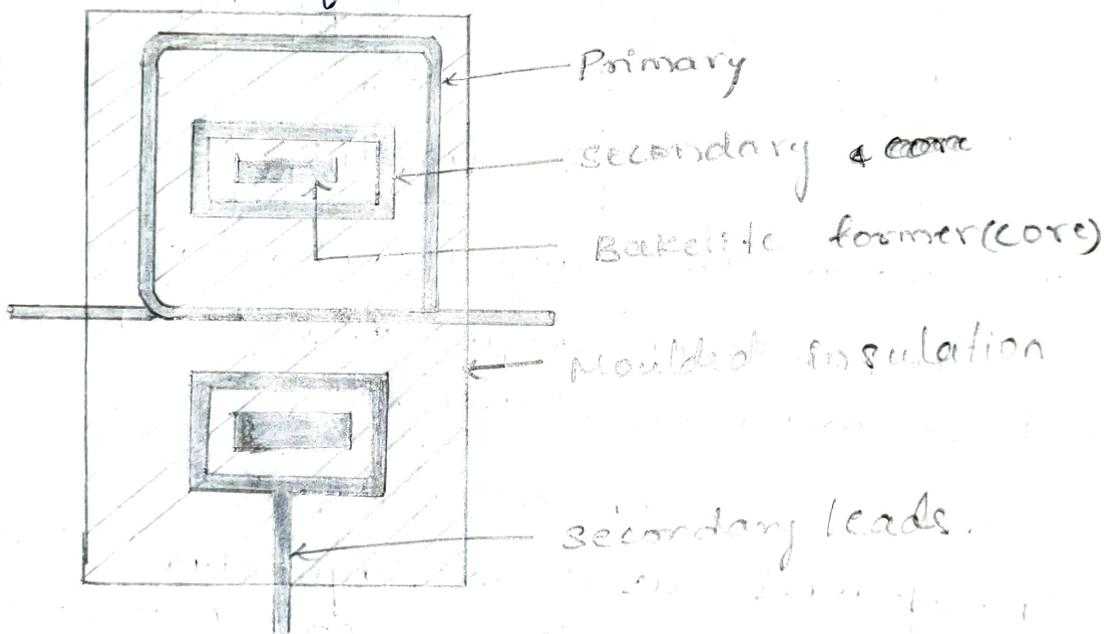
\* In a low voltage wound type C.T secondary winding is wound on bakelite former. heavy primary winding is wound on secondary winding with suitable insulation in between or
