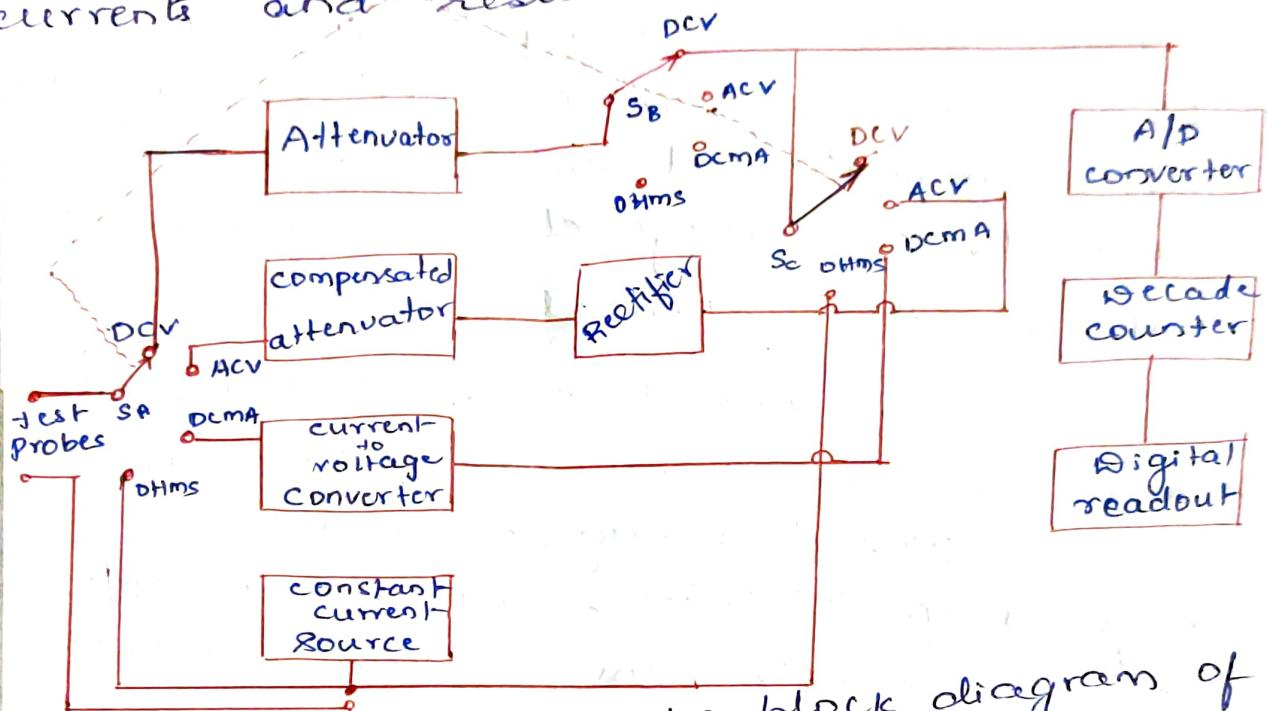
Above fig shows the block diagram of digital multimeter.
