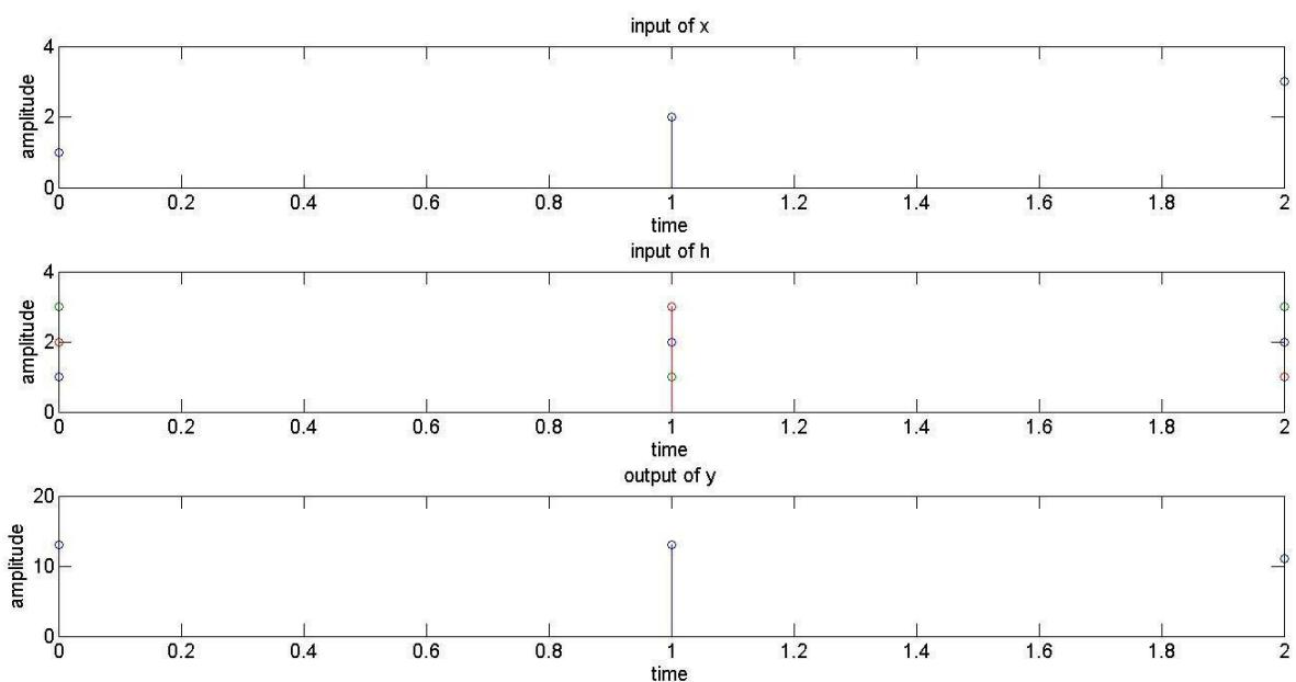
c) linear convolution from circular convolution with zero padding.
