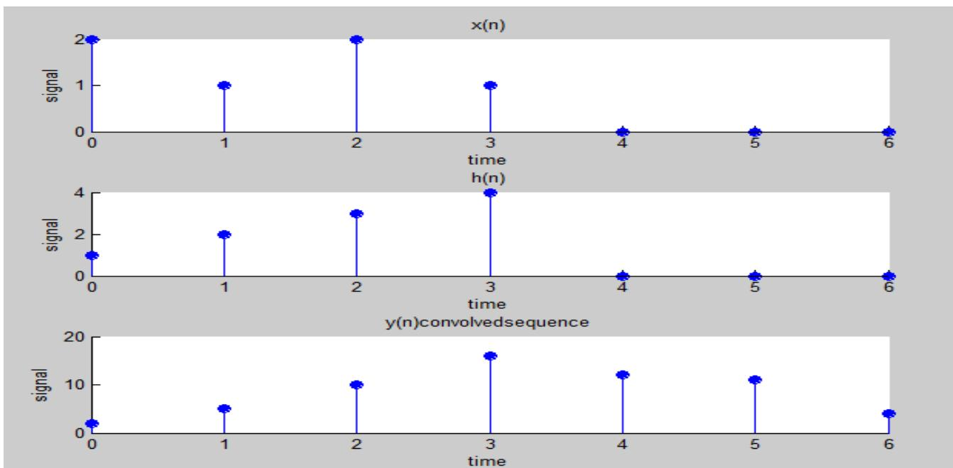
**b. Circular convolution using DFT and IDFT method**
