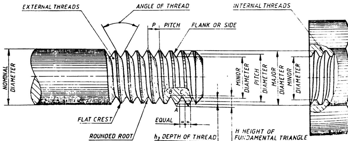
Elements of a Screw Thread
