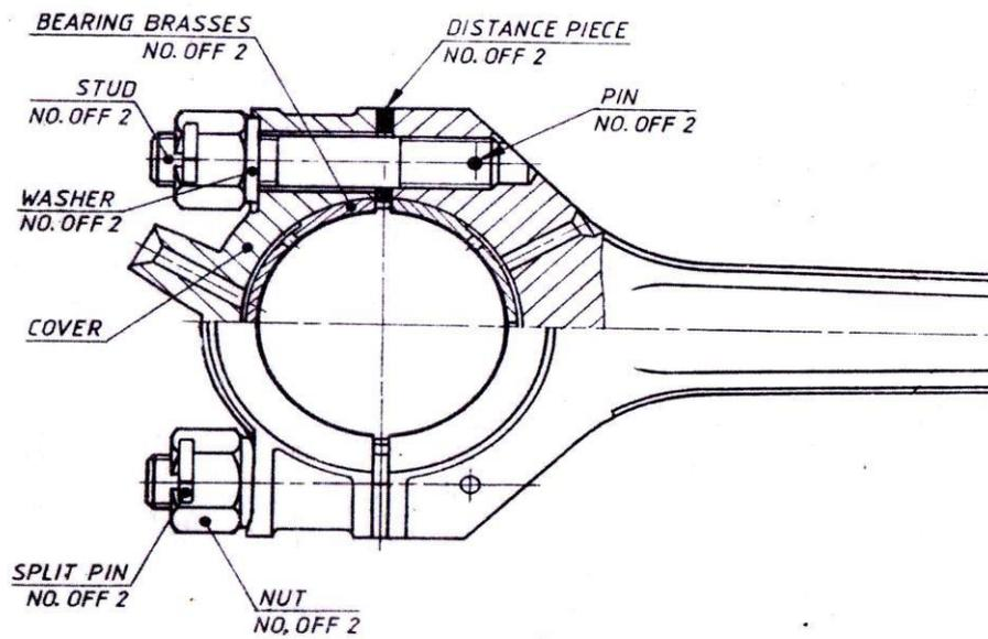
Fig. shows the details of a PETROL ENGINE CONNECTING ROD. Draw the following assembled views of the connecting rod with its axis horizontal to 2:1 scale.
