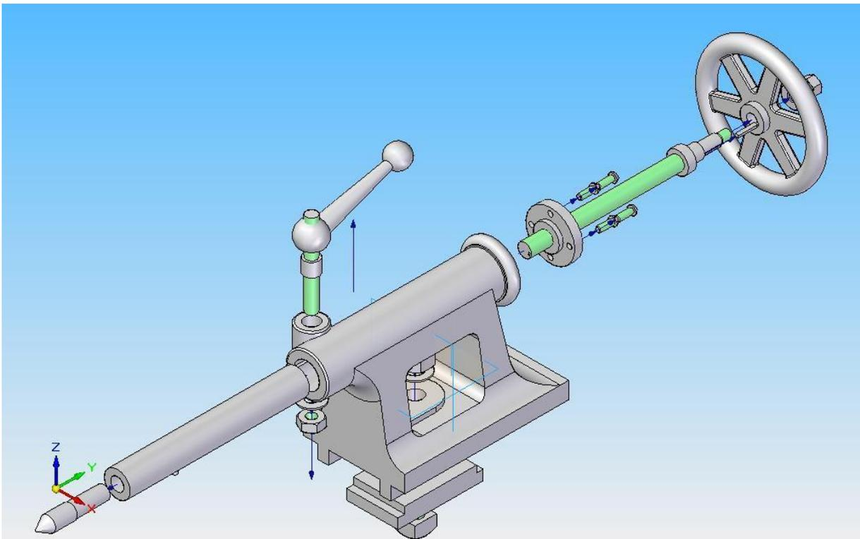
Figure shows the details of a tail stock of a lathe. Assemble the parts and draw
