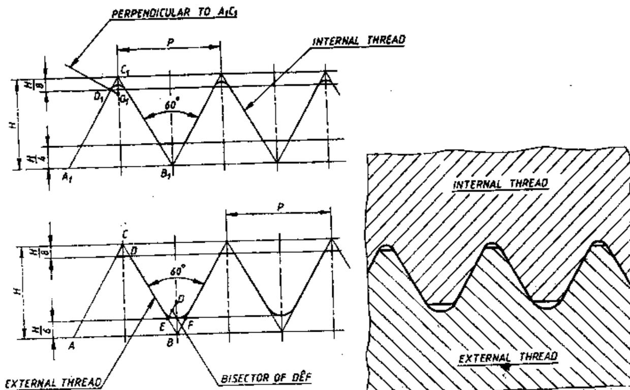
**Whitworth Thread (British Standard) BSW Threads**
