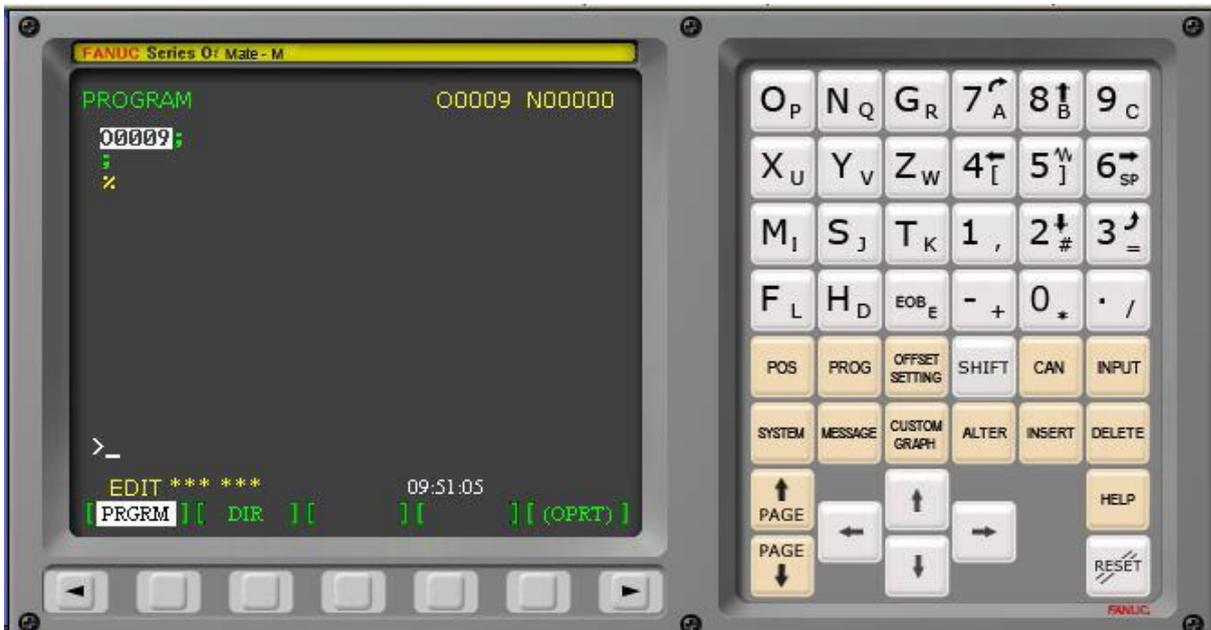
Type the program by using Program panel or by using the computer key board .
