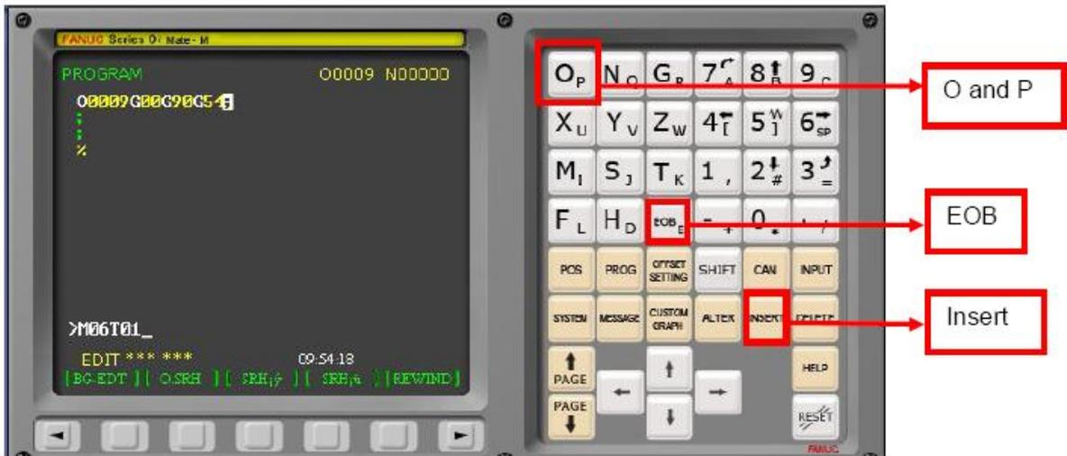
In program panel press letter in smaller font press **Shift** then press button for example to type letter p press **Shift** then press **O and P** Button. After entering one line of code press **EOB** button press **Insert** button add this code to numerical control panel.
