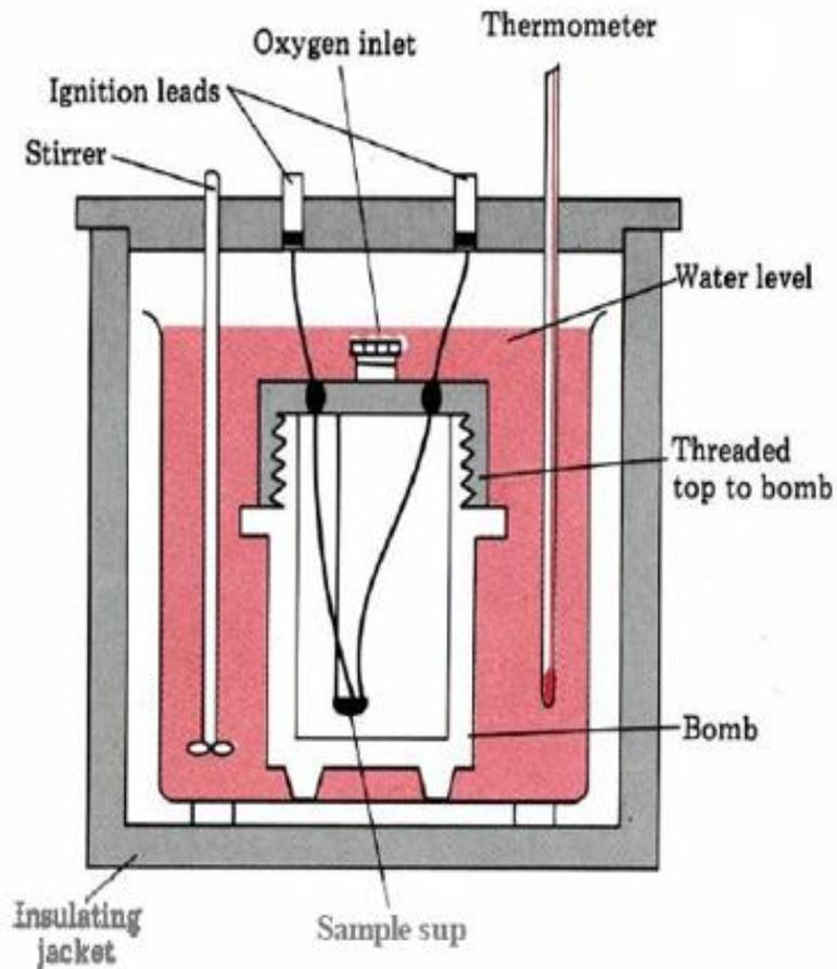
**Fig. Bomb Calorimeter**
