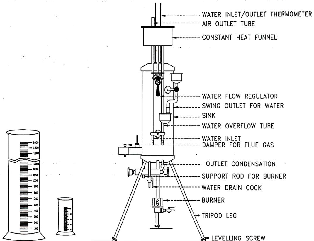
**Introduction:** This calorimeter is intended for the purpose of determining the “Calorific value of gaseous fuel” experimentally. The method is based on heat transfer from burning the known quantity of gaseous fuel for heating the known quantity of water that circulates in a copper coil heat
