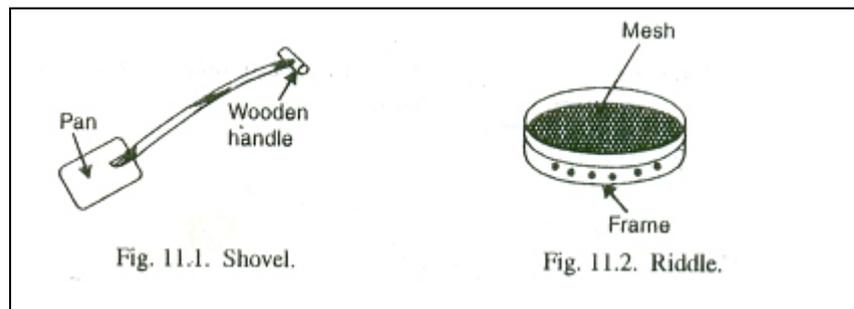
2. **Riddle:** A riddle, as shown in Fig. 11.2, has a standard wire mesh fixed into a circular or square wooden frame. It is used for cleaning the moulding sand. The riddles are specified by the diameter of the frame and the mesh number. When large volumes of sand are to be cleaned, then power operated riddles are used.
