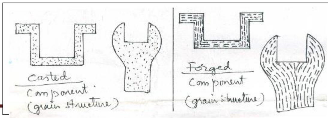
The basic rule of obtaining a forged and casted component is that in a forged component the grains are arranged radially thus increasing the resistance to shock. A casted component has a symmetrically aligned grain arrangement and is thus weaker as compared to forged component.
