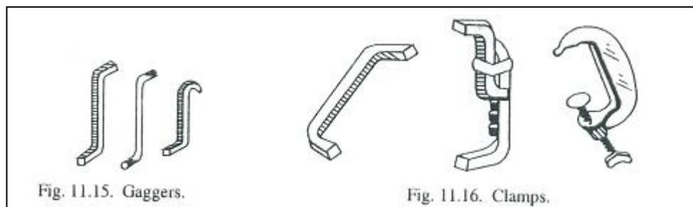
15. **Gagers:** the gagers (also called lifters), as shown in Fig. 11.15, are iron rods bent at one end or both ends. It is used for reinforcement of sand in the top part of a moulding box and to support hanging bodies of sand. The length of the gagers vary from 125 mm to 600 mm and they are coated with clay wash to cause the sand to adhere to them.
