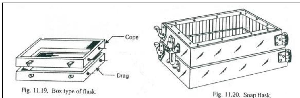
These flasks should not be removed till the pouring of molten metal is completed. Hence a number of tight flasks are required for any one moulding sets up, one for each mould being processed. These flasks are generally made of steel.
