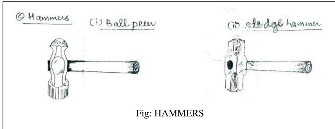
The hammers commonly used in hand forging are:-
