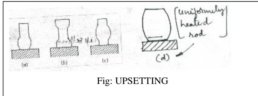
It is the process of increasing the cross section of a bar at the expense of its length.
