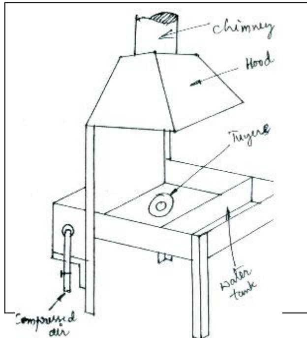
A smith's forge or hearth is used to heat the metal to be shaped.
