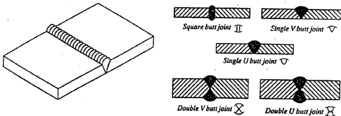
Fig. 18 Butt welds
