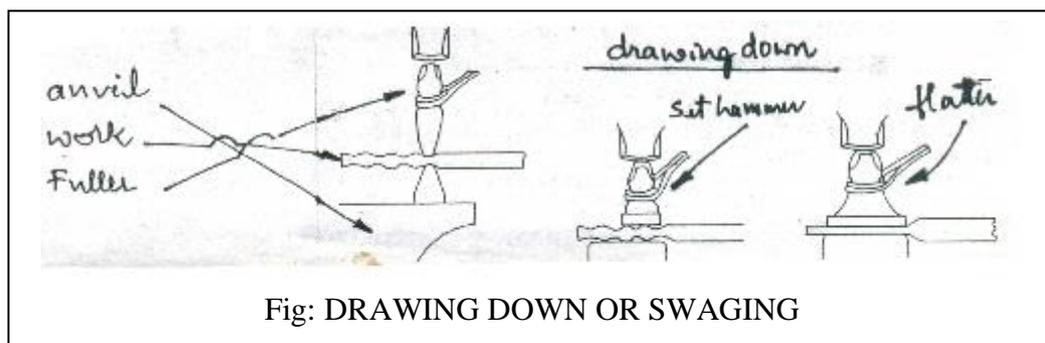
It is the process of reducing the cross-section of a bar and increasing its length.
