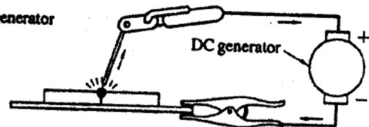
Fig. 3 Reverse polarity
