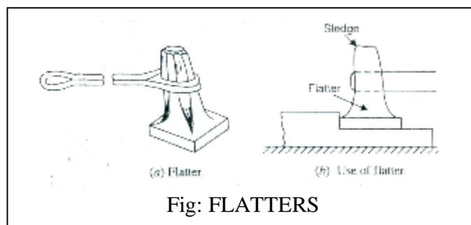
1. The flatter is used for finishing flat surfaces and are made with a perfectly flat face.
