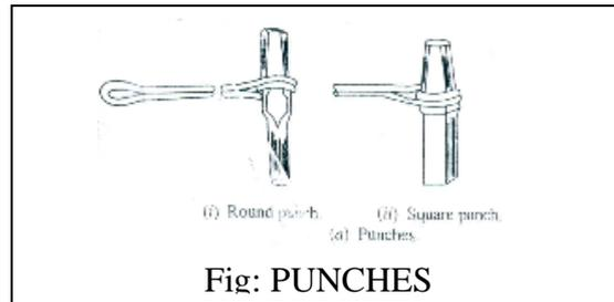
1. These are used for making holes when the metal is at forging heat.
