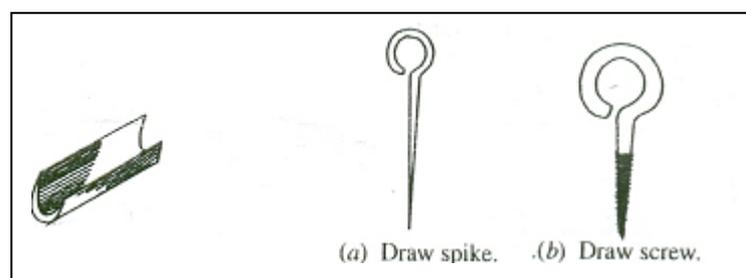
11. **Draw spike and screw:** A draw spike, as shown in Fig. 11.11(a), is a pointed steel rod, with a loop at one end. It is driven into a wooden pattern to hold it when the sand is withdrawn. The draw screw, as shown in Fig. 11.11(b), is similar in shape but threaded on the end to engage metal patterns.
