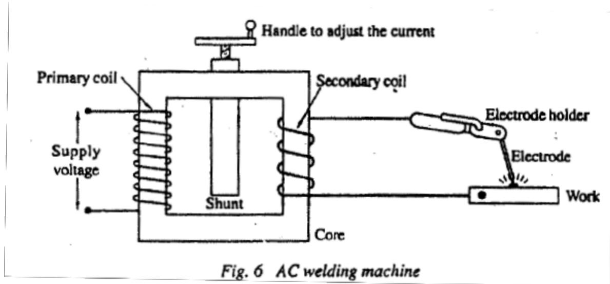
**AC transformer welding machine:** Fig.6 illustrates transformer type AC welding machine. The function of the transformer is to step down the voltage and to generate high amperage current required for welding. It consists of a square block-shaped core, a primary coil, which carries the input current, and a secondary coil which is connected to the electrode holder. A movable shunt between the two coils controls the secondary coil current (welding current).
