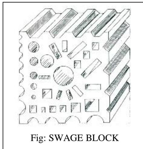
1. Swage block, is generally made of cast iron and has round, square, rectangular and half-round grooves
