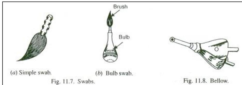
A bulb swab, as shown in Fig. 11.7(b), has a rubber bulb to hold the water and a soft hair brush at the open end. It is used for moistening the sand around the edge before the pattern is removed.
