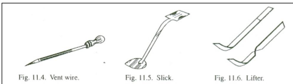
5. **Slick:** A slick, as shown in Fig. 11.5, is a small double ended tool having a flat on one end and a spoon on the other. This tool is also made in a variety of other shapes and is used for repairing and finishing the mould surfaces after the pattern is withdrawn.
