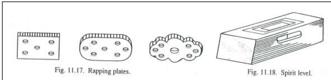
19. **Spirit level:** A spirit level, as shown in Fig. 11.18, consists of an air bubble in a curved glass tube protected by a wooden or metal frame. It is used by the moulder to ensure that his bed of sand, moulding box or moulding machine table is horizontal.
