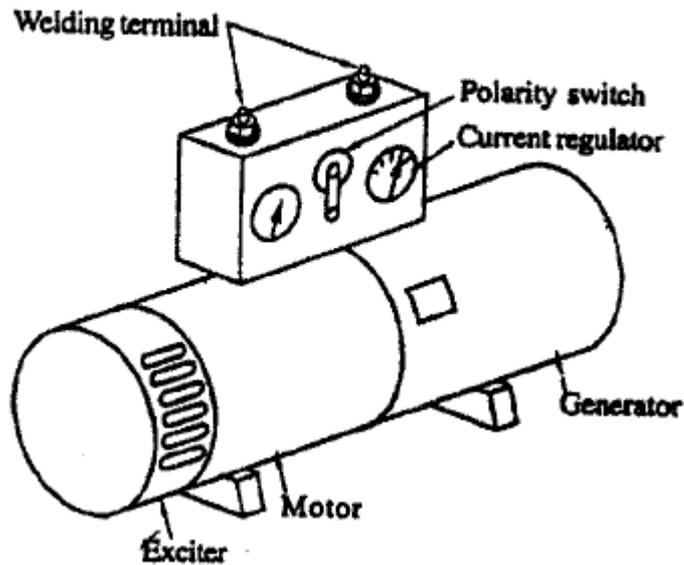
Fig. 7 DC motor-generator welding machines
