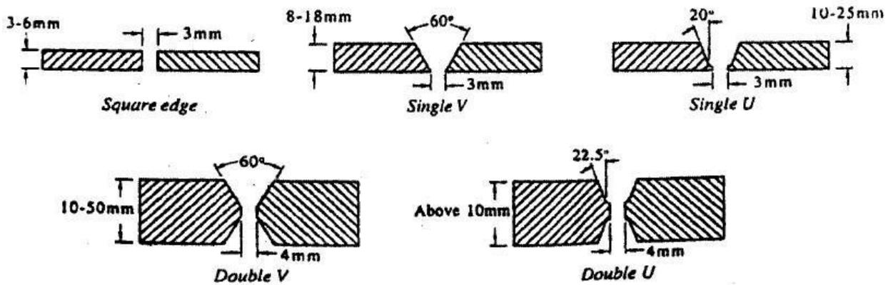
Fig. 23 Edge preparation of butt joint
