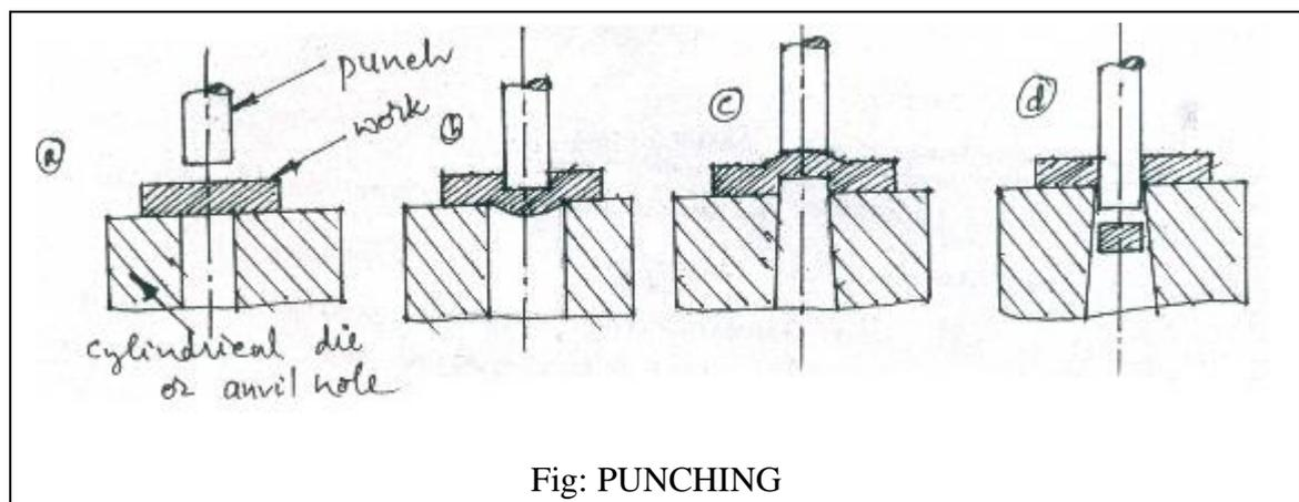
It is the process of producing holes by forcing the punch through the work. The work may be placed over the pritchel hole of the anvil, over a cylindrical die, over a hole of correct size in the swage block.
