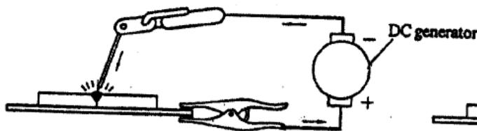
Fig.2 Straight polarity
