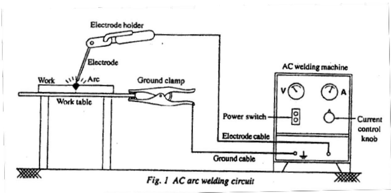
Fig. 1 AC arc welding circuit
