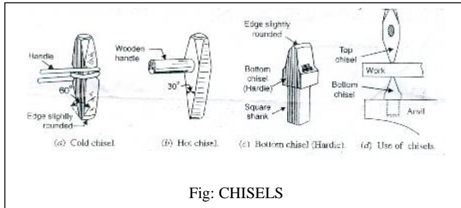
Chisels are used for cutting metals and for necking prior to breaking. They may be cold or hot depending upon whether the metal to be cut is cold or hot. The main difference between the two chisels is in the edge.
