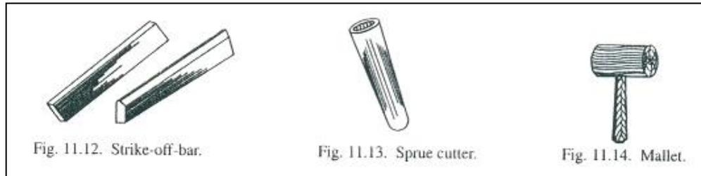
13. **Sprue cutter:** A sprue cutter (also called a runner peg), as shown in Fig. 11.13, is a tapered wooden peg. It is forced into the top part of the mould (known as cope) at the correct position. When the peg is withdrawn, it leaves a cavity (known as down gate) through which the molten metal is poured.
