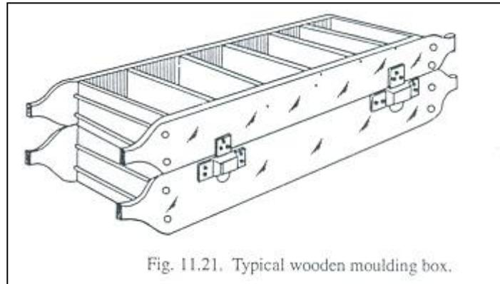
A typical wooden moulding box is shown in Fig. 11.21. The side timbers are continued beyond the ends of the box to form two handles at each end. The sides are held together by strong cross timbers, reinforced with bolts. The crossbars prevent the sand from falling out when the top part of the box (i.e., cope) has been rammed up and is lifted away from the bottom part of the box (i.e., drag).
