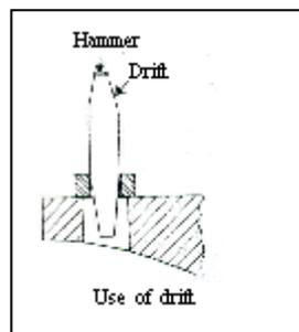
1. The drift is used to finish the size of the punched holes.
