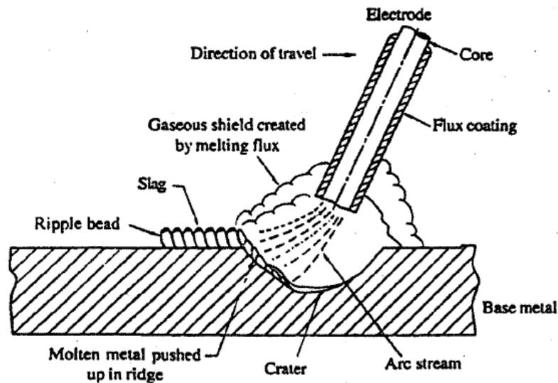
Fig. 5 Shielded metal arc welding
