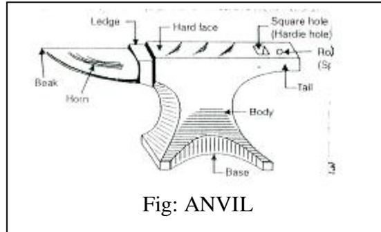
1. The anvil forms a support for blacksmith's work when hammering.
