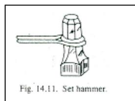
1. The set hammer is similar to flatter, but is a smaller tool. It is made up of forged steel and is hardened.
