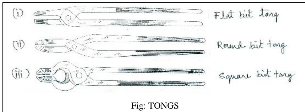
Tongs are used for handle the work while forging. These are made of mild steel and sizes vary from 40cm to 60cm in length and 0.6cm to 5.5cm opening.
