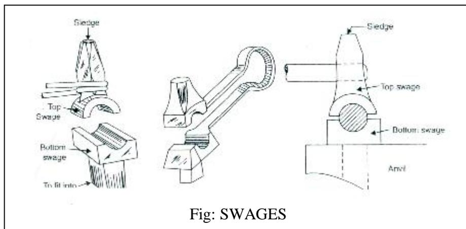
1. The swages are used for work which has to be reduced and finished to round or hexagonal form.
