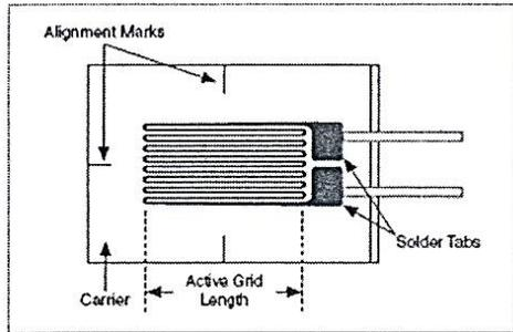
Fig.1.1 a. Strain gauge beam
