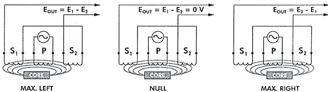
Fig.3.2. Three different cases of LVDT core position
