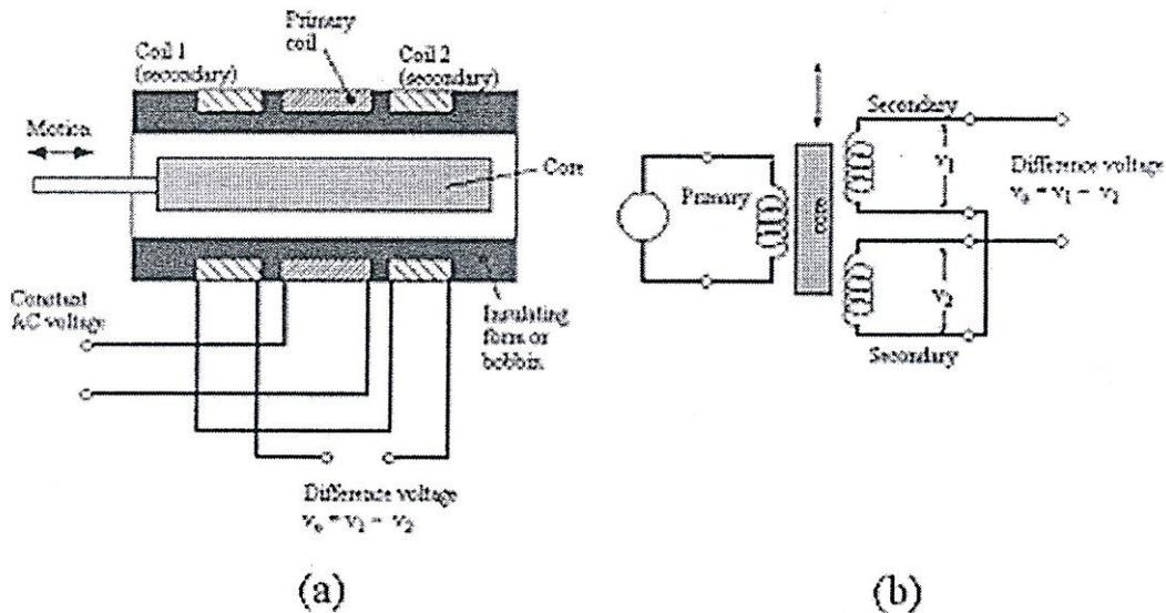
Fig.3.1. Schematic diagram of LVDT
