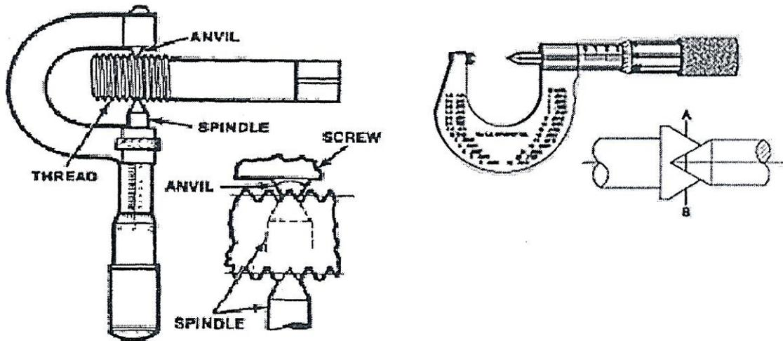
Fig.11.3. Screw thread micrometer
