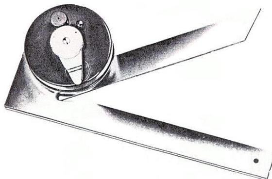
Fig.6.2. Optical bevel protractor
