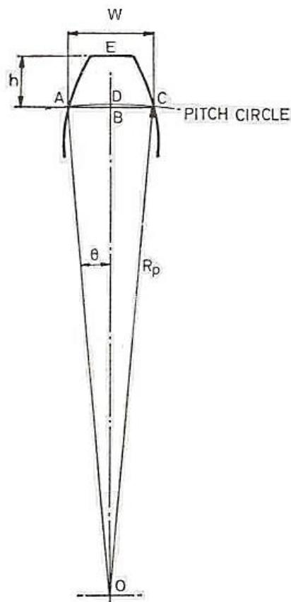
Fig.7.3. Measurement of tooth thickness at pitch circle diameter
