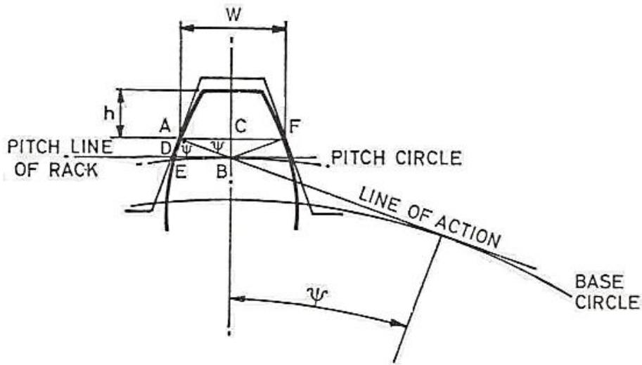
Fig.7.4. Measurement of tooth thickness at constant chord
