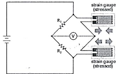
Fig.1.1 d. half bridge connection
