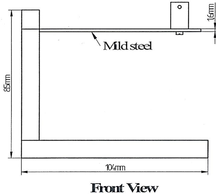
Fig.1.2. Strain gauge cantilever jig
