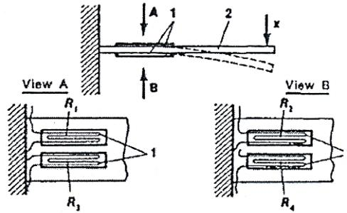
Fig.1.1 b. Strain gauge attached to cantilever beam
