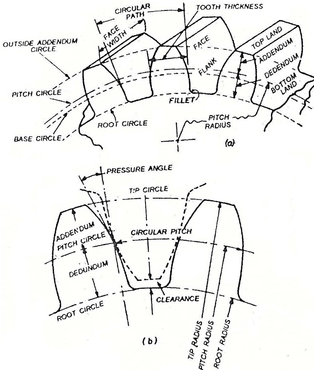
Fig.7.2. Spur gear tooth gear
