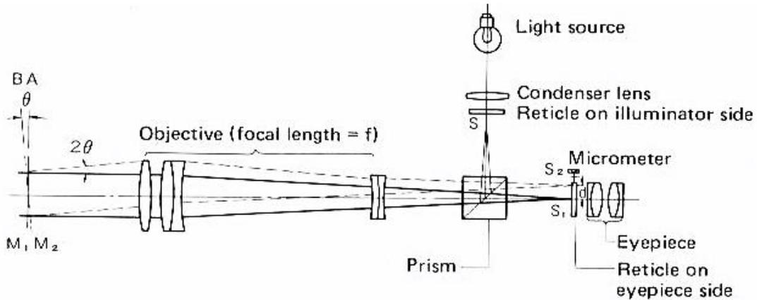
Fig.10.1. Working principle of Autocollimator
