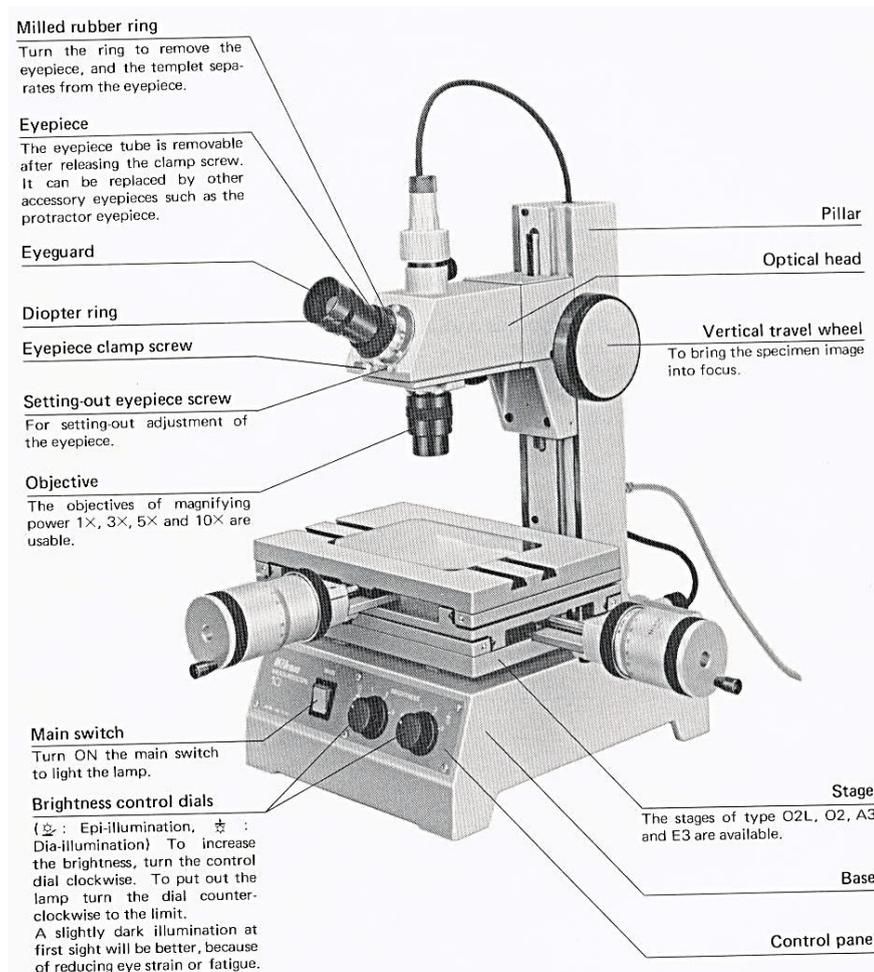
Fig.9.1 Tool maker's microscope (Measroscope)
