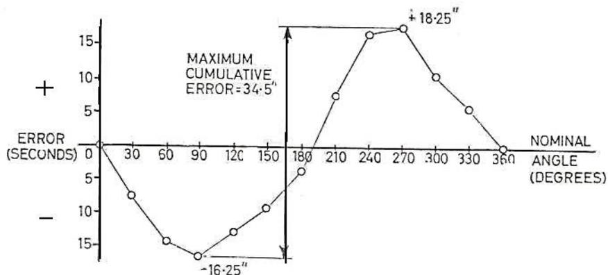
Graph of indexing errors from an indexing device having an eccentric mounting.
