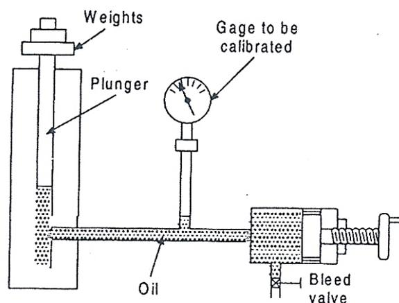
Fig4.2. Dead weight pressure gauge
