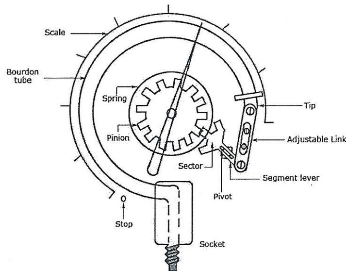
Fig 4.1. Bourdon tube pressure gauge
