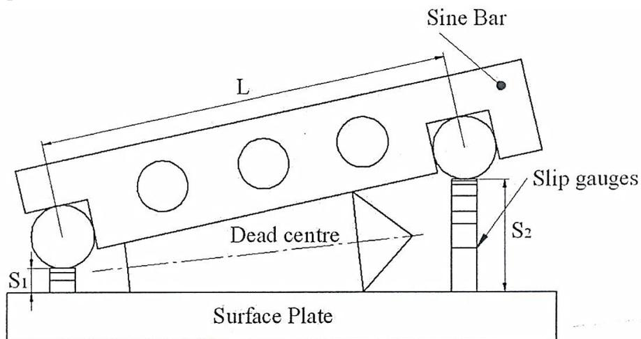
Fig.6.1. Experimental setup to measure taper angle using Sine bar
