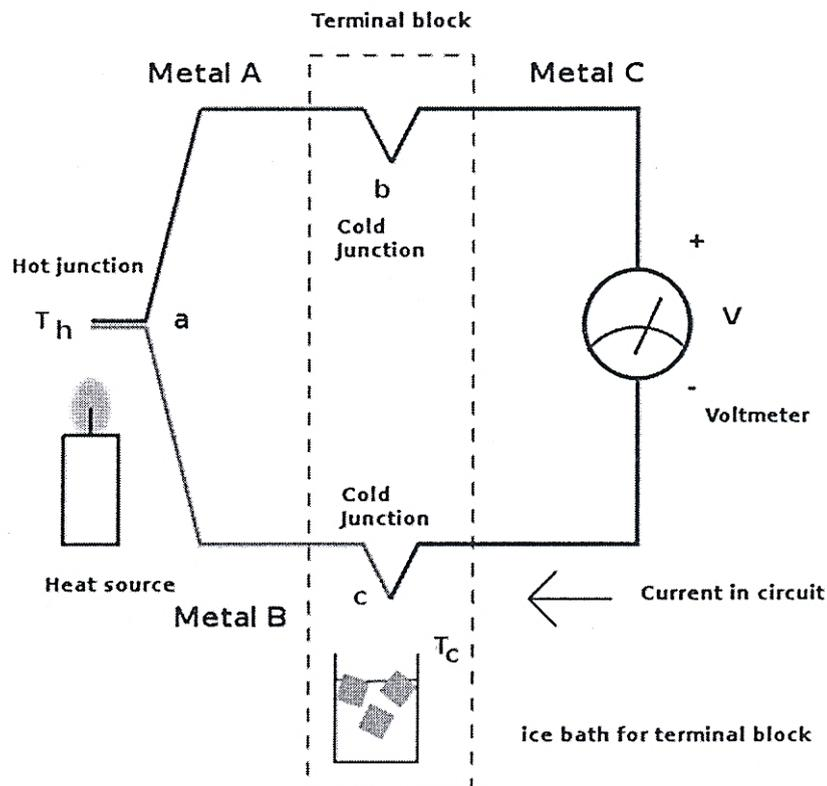
Fig. 2.1 Temperature measuring circuit using Thermocouple
