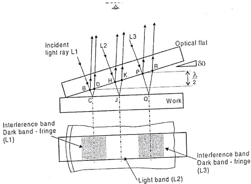
Fig.13.1. Fringe generation by interference
