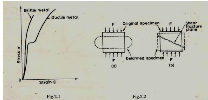
the specimen is too long. The engineering stress-strain curve for brittle and ductile material in compression test are shown in fig.2.1
