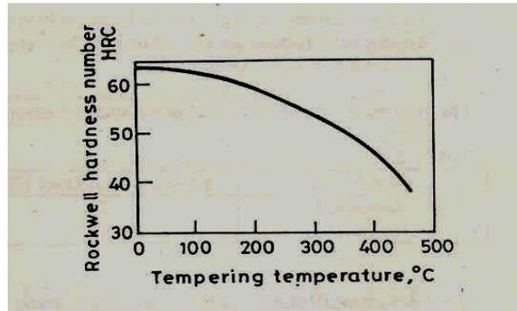
Fig. shows the variation of Rockwell C hardness number with increase in temperature.
