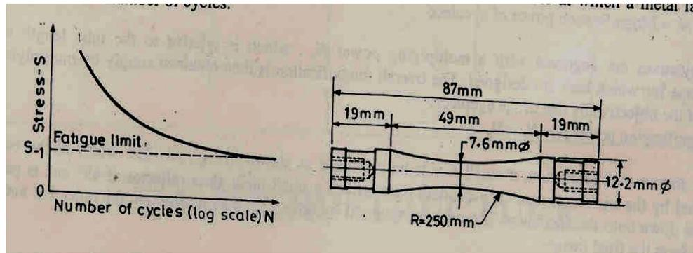
**Specimens:** All specimens should be taken from the same rod, each specimen should receive same kind of machining and heat treatment. The specimens for tests of the metal have no sharp stress raisers. The surface of the specimen is polished. The standard specimen for rotating beam test is shown in Fig. 10.4.
