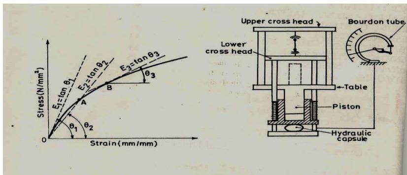
Universal testing machines (UTM) are used for tension compression, bending, and transverse shear tests. UTM are generally either of the screw-gear or hydraulic type. Fig. 1.4 shows the essential features of the universal hydraulic machine. A motor driven pump is used to transmit oil to cylinder, thereby producing pressure against a piston. The pressure transmits a force to the tensile specimen by means of upper cross head. The adjustable lower cross head can be moved up or down
