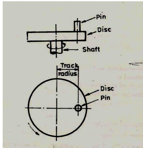
Fig.6.1 pin-on-disc type wear-testing machine
