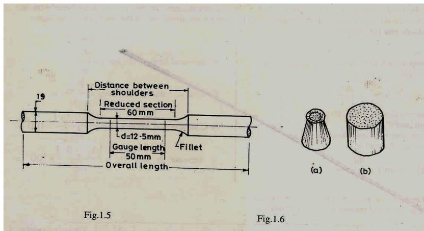
**Fracture appearance:** The fracture of mild steel in the form of standard cylindrical specimen usually has a cup-cone type of silky texture as shown in fig. 1.6(a). The typical fracture of cast iron is gray, flat and granular as shown in fig. 1.6(b).
