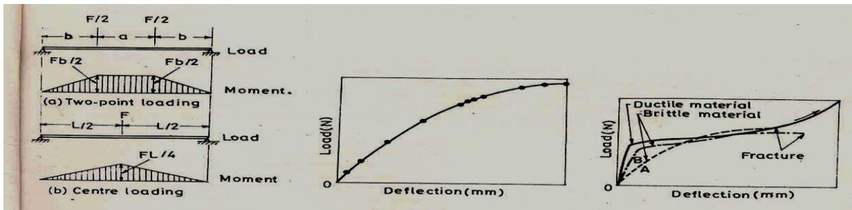
Fig.5.1 specimens subjected to load
