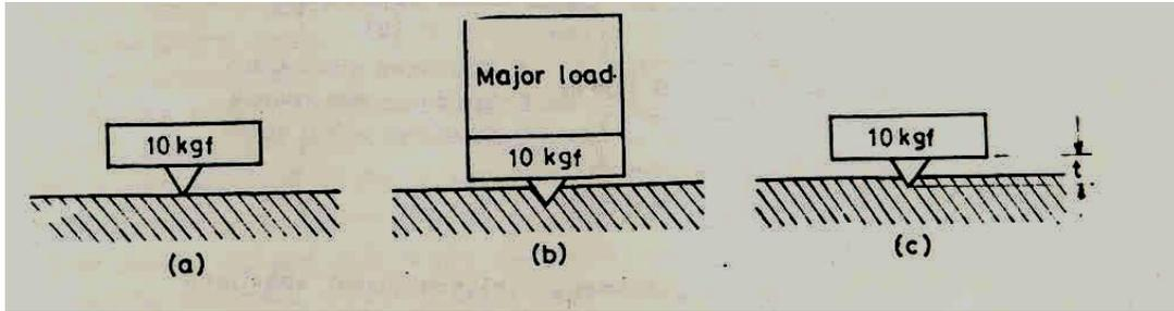
Fig. stages of Rockwell hardness tests.
