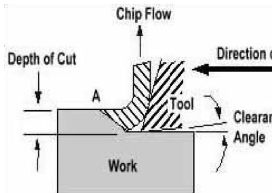
Figure 1: Basic Metal Cutting Theory against the tool.
