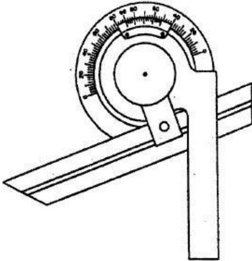
Fig. 8 Bevel Protractor
