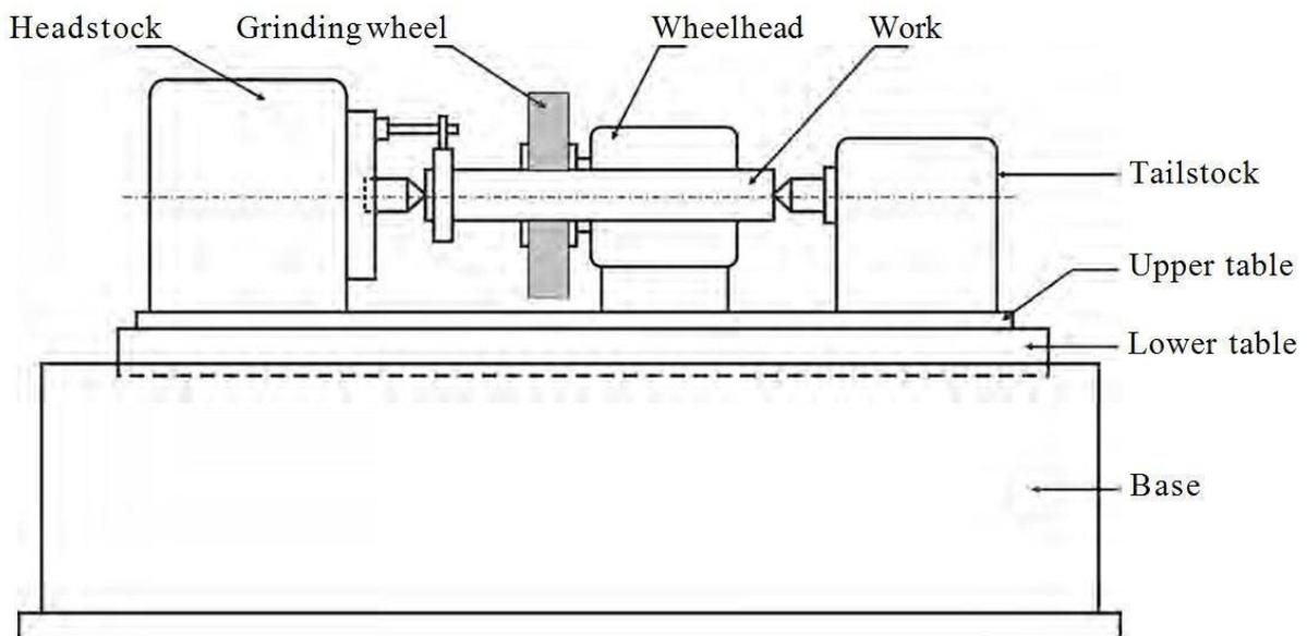
Figure 29: Cylindrical Grindin Machine
