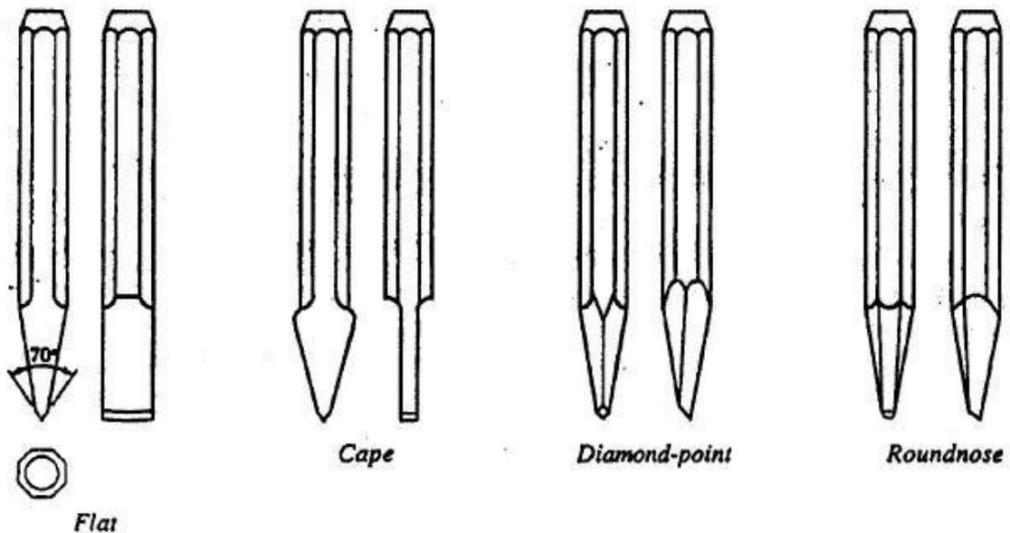
Fig. 30 Type of cold chisels
