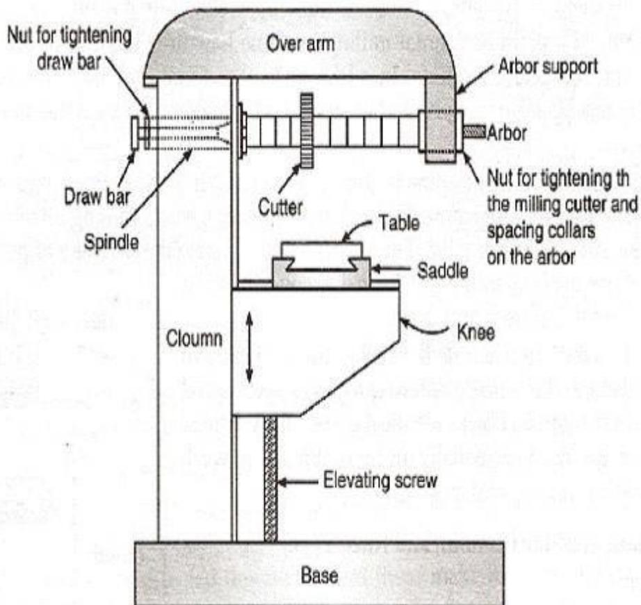
Figure 19: Column and Knee type Milling Machines
