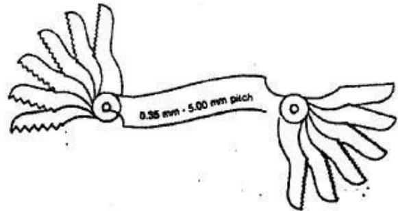
Fig. 9 Screw-pitch gauge
