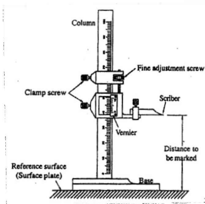
Fig. 20 Vernier height gauge
