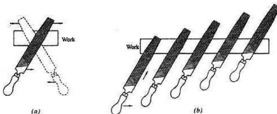
Fig. 39 Method of holding a file
