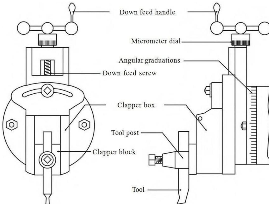
Figure 14: Shaper Tool Head
