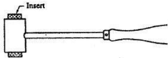
Fig. 29 Soft-faced hammer
