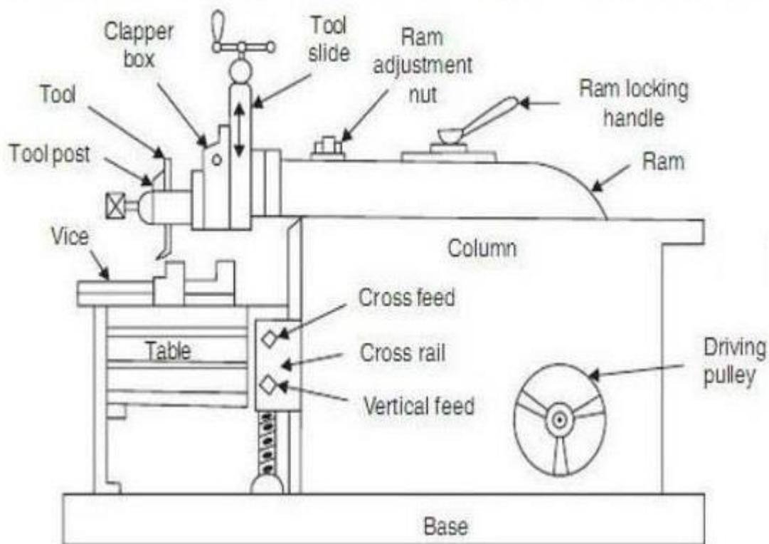
Figure 13: Standard Shaping Machine
