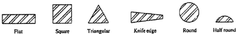
Fig. 35 Cross sectional shapes of common files
