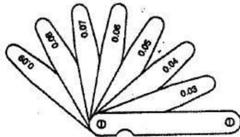
Fig. 10 Thickness gauge
