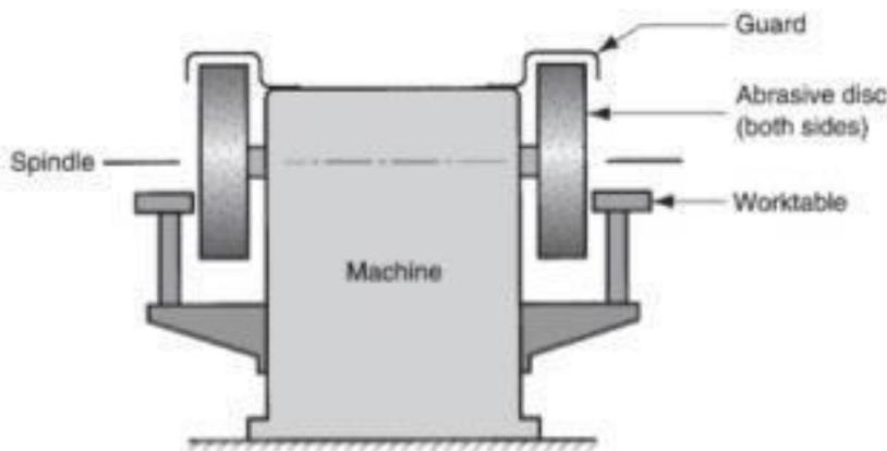
Figure 28: Bench Grinding Machine
