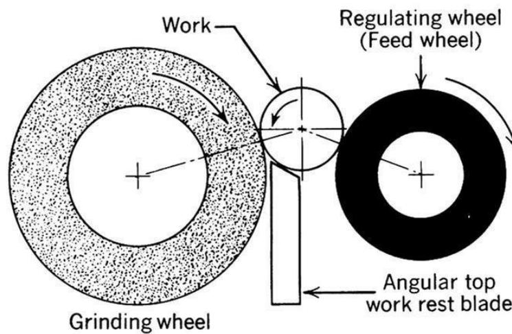
Figure 30: Centreless grinding mechanism
