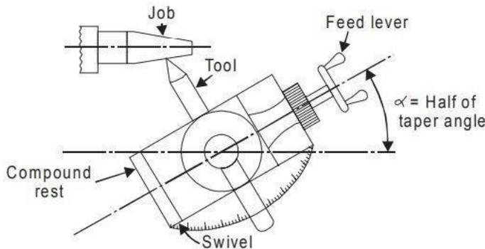
Figure 9: Taper turning by swiveling compound rest
