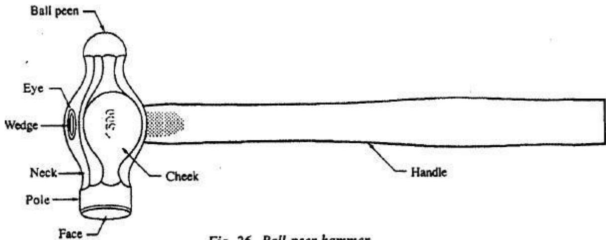
**Fig. 26 Ball-peen hammer**
