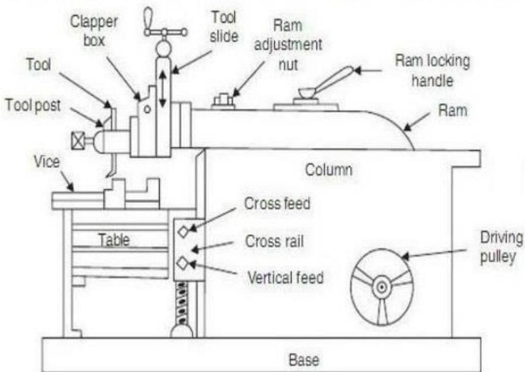
Figure 13: Standard Shaping Machine
