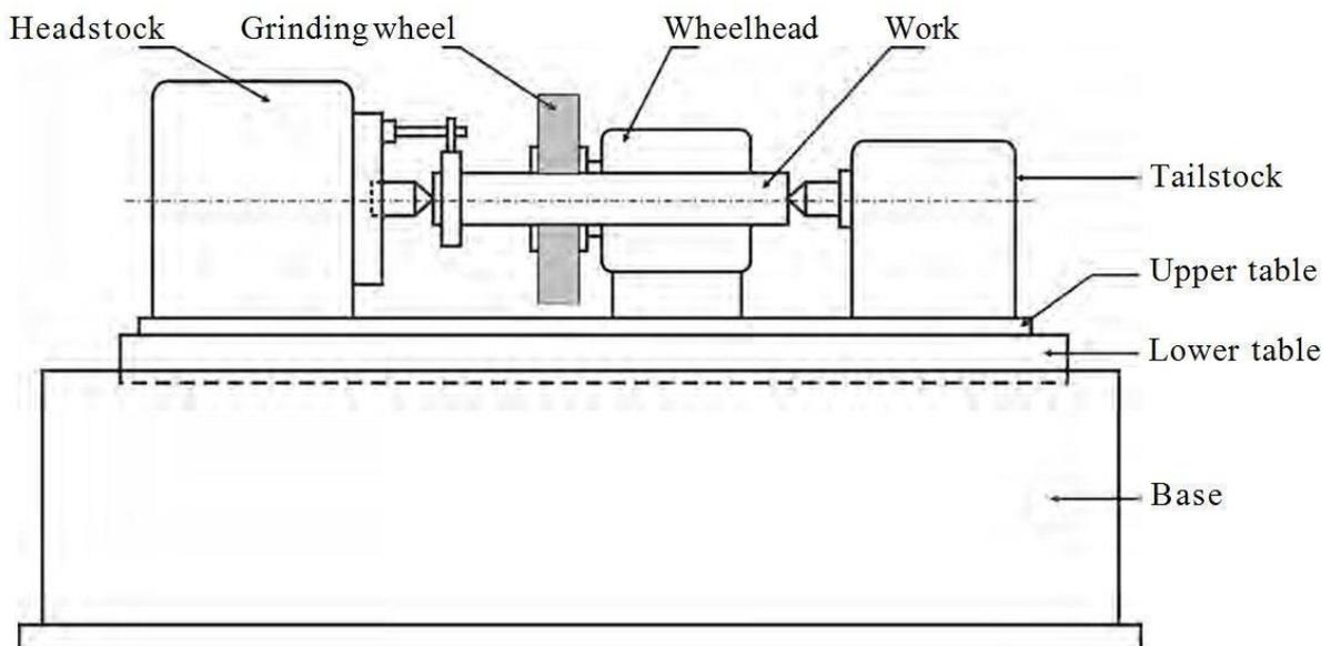
Figure 29: Cylindrical Grindin Machine
