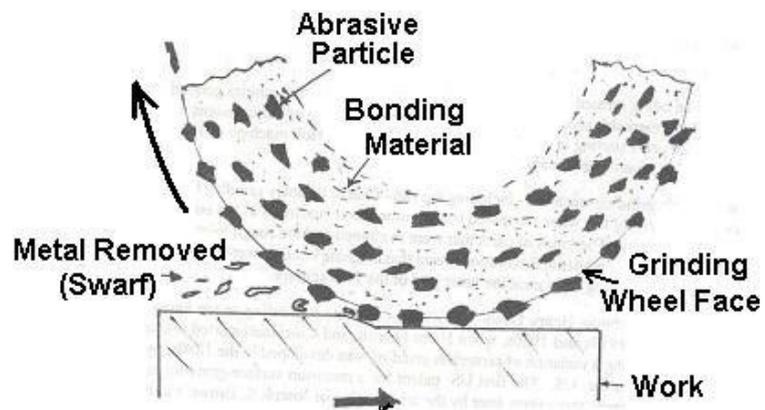
Figure 31: working principle of Grinding Wheel
