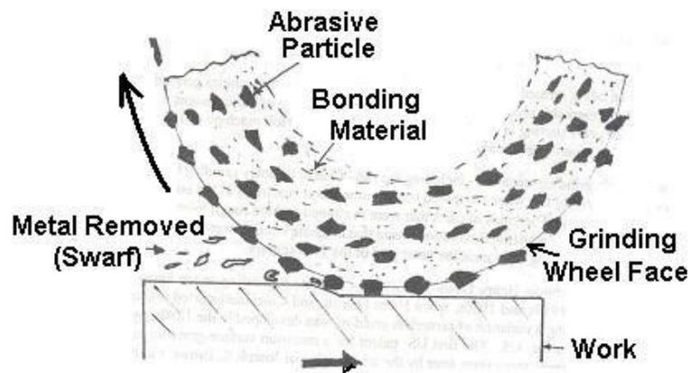
Figure 31: working principle of Grinding Wheel
