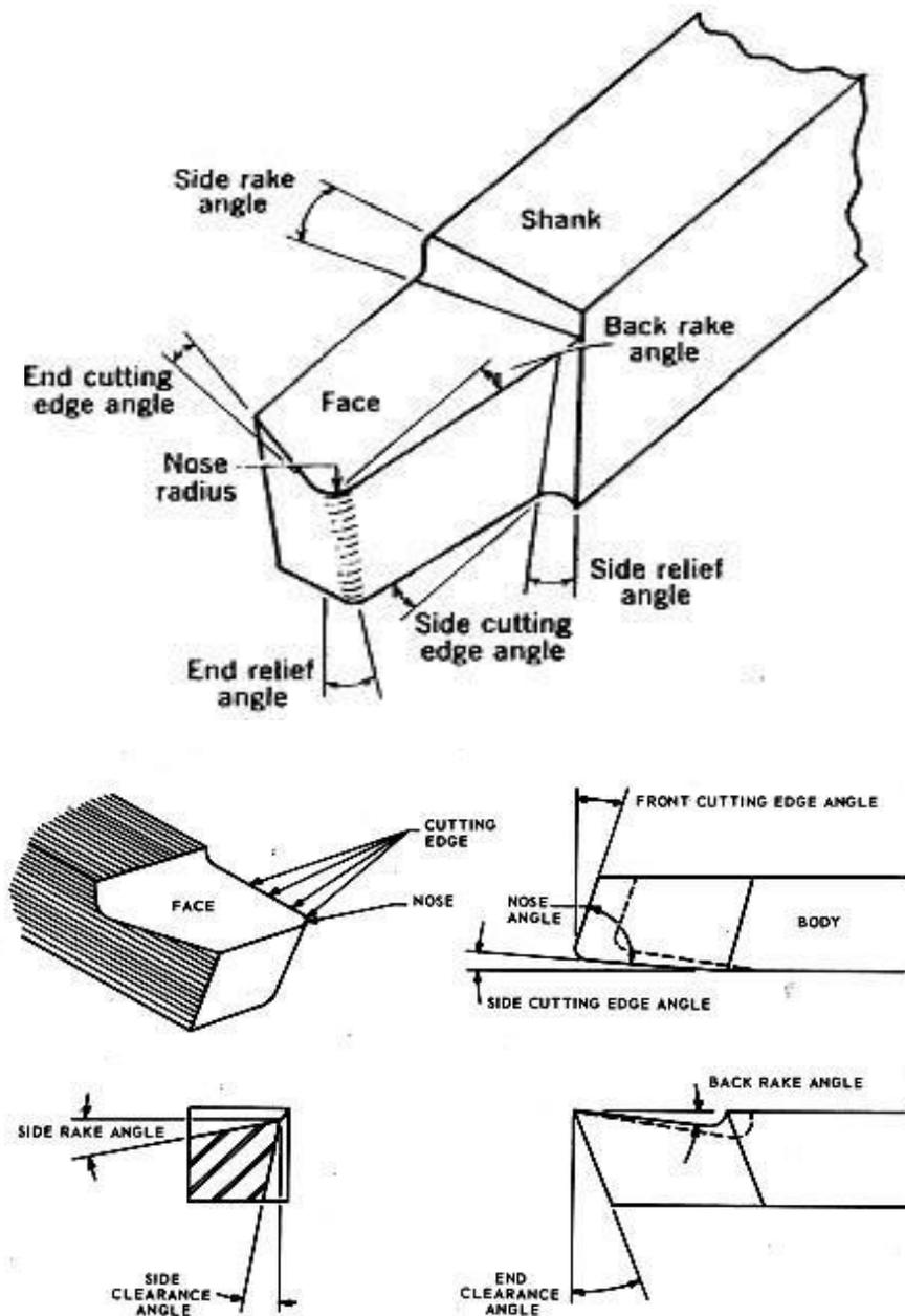
Figure 2 Cutting Tool Terminology
