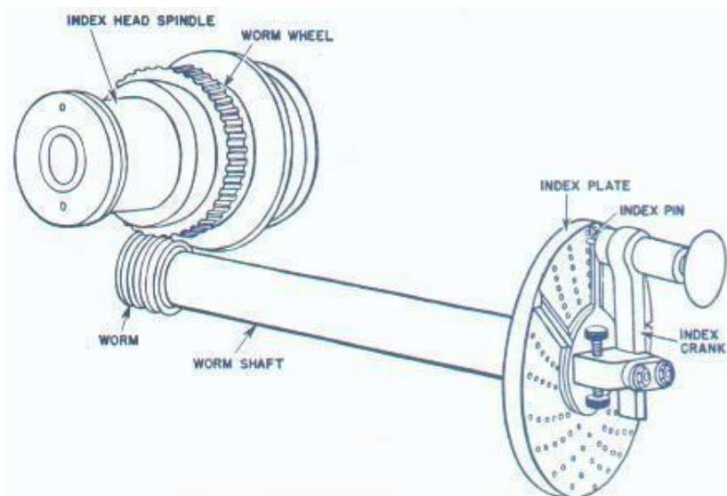
Figure 26: Simple Indexing Mechanism
