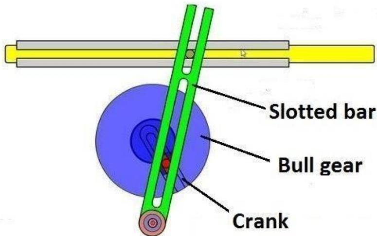
Figure 16: Crank and slotted link mechanism
