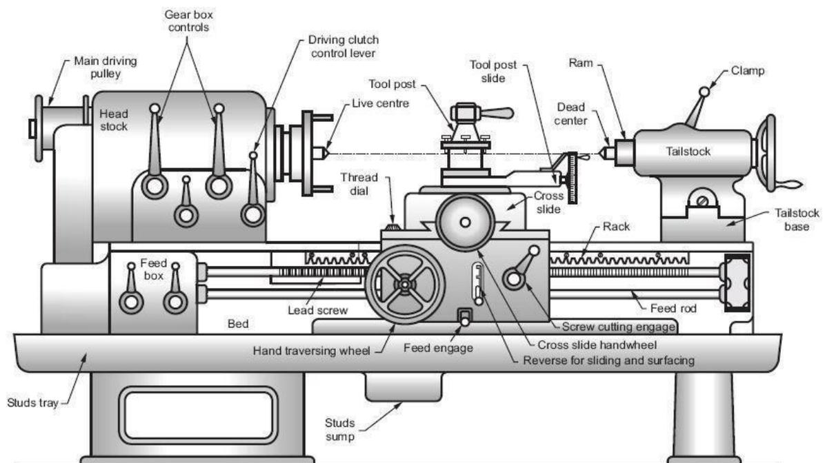
Figure 4: Different parts of engine lathe or central lathe
