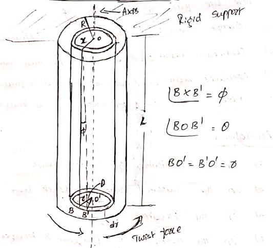
Consider a long cylindrical rod of length  $L$  and radius  $R$ , rigidly fixed at its upper end. Let  $OO'$  be axis of cylindrical rod.
