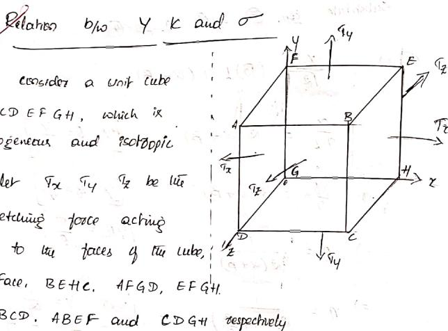
If  $\beta$  is coefficient of compression, i.e. contraction produced per unit length per unit tension to the direction perpendicular to the forces. Then contraction produced in the perpendicular to the edges AB, BE and BC will be  $T_x \beta$ ,  $T_y \beta$  and  $T_z \beta$ .
