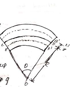
If we loaded at N the successive layers are strained such that AB is elongated to A'B' & EF is contracted to E'F' & CD is remains unchanged (neutral surface) which is as shown in the fig.
