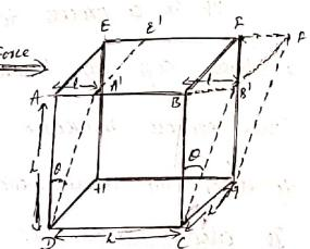
It is defined as the ratio of the relative displacement b/w the two layers, under the action of a tangential force, to the distance b/w them, the distance being measured at right angles to the direction of stress.
