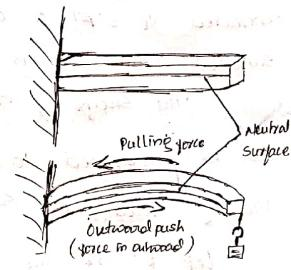
These two groups of forces result in a restoring couple, which balances the applied couple, acting on the beam.
