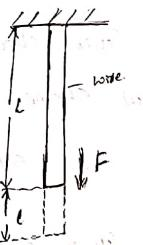
The applied force per unit area of cross section along normally, which is called "Longitudinal stress".
