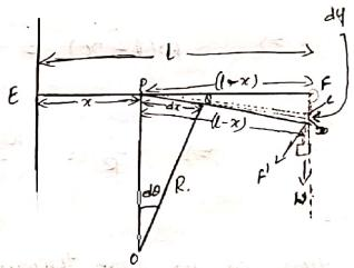
Bending moment = Force  $\times$  perpendicular distance.
